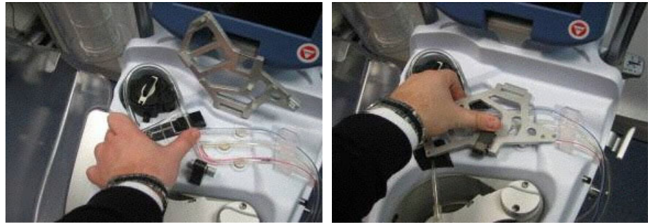
Figure 4-8 Seating the Pump Loop Cartridge (Left); Latching the Clamp Lid (Right)
