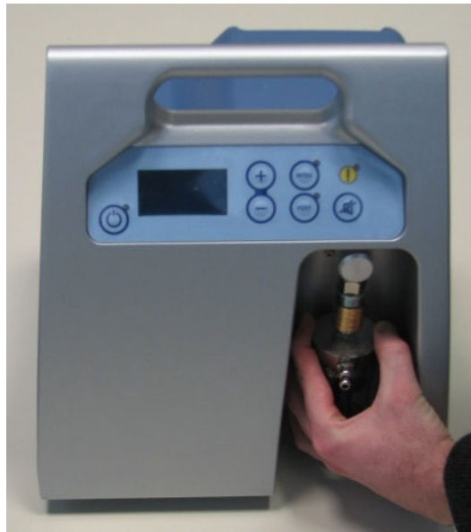
Figure 15-4 Removal of the Overflow Trap from the Vacuum Pump
