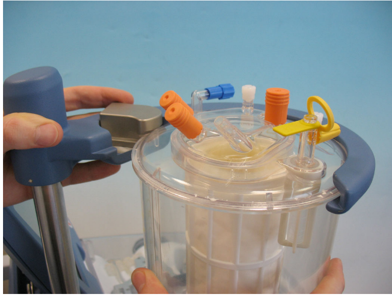
Figure 4-2 Positioning the Blood Collection Reservoir on the Reservoir Holder
