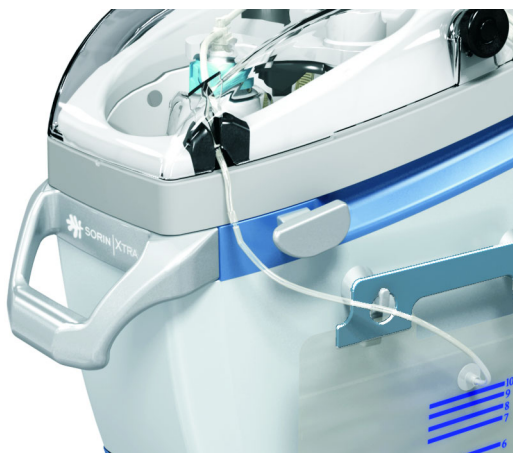
Figure 4-12 Connecting the Waste Bag
