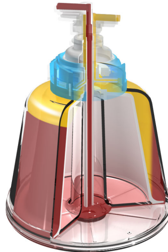
Figure 3-32 Cross-Section of Latham Centrifuge Bowl
