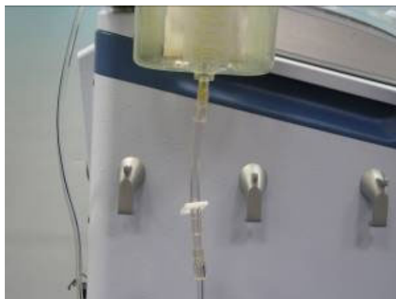
Figure 4-10 Connecting the Bowl Set to the Bottom of the Blood Collection Reservoir
